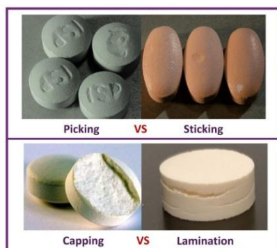
Fig. 3: Shown different manufacturing challenges.
