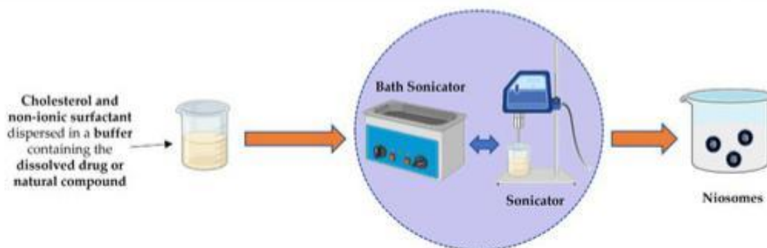
Figure 5: Sonication Method (Adapted from 12)
