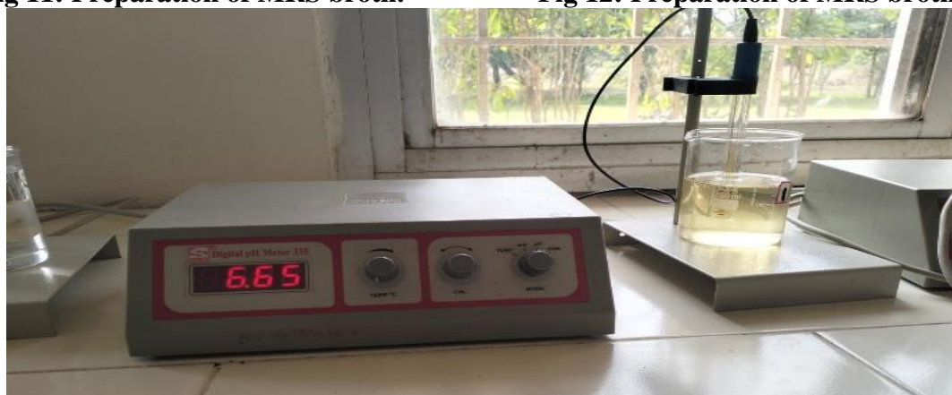
Fig 13: Measurement and adjustment of the final PH of MRS broth medium. The medium was adjusted to 6,65 using 0.1N NAOH for the growth of lactic acid bacteria.
