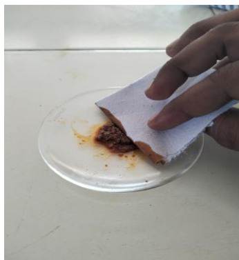
Fig 3: Oil separation from pickle.
