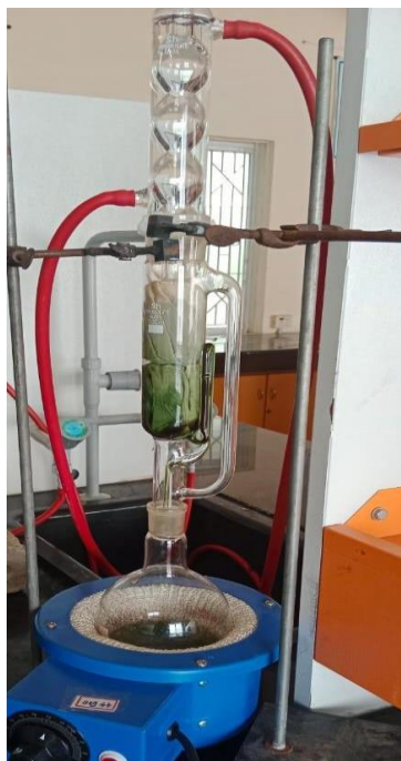
Figure 2: Soxhlet Apparatus Extraction.
