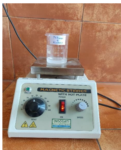
Fig 4.5: - Mixing polymer using magnetic stirrer.
