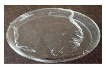
**Justification:** Plasticizer was too low, and film dried excessively fast, sticking hard to the surface and tearing during removal.
