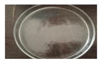
**Justification:** Lower polymer caused weak matrix; although plasticizer was optimum, the film retained moisture and stayed gel-like even after drying.
