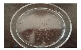
**Justification:** Reduce polymer and higher plasticizer increased film flexibility but trapped air during casting, causing visible bubbles.
