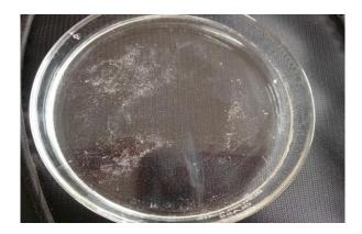
**Justification:** Improper dispersion or incomplete solubility of HPMC E15 in the solvent led to white patches.
