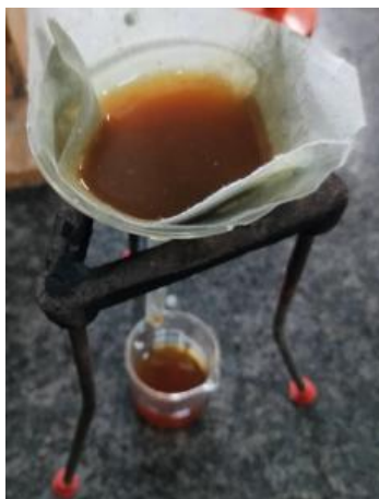
Fig. 9: Filtration of Mulethi Extract.
