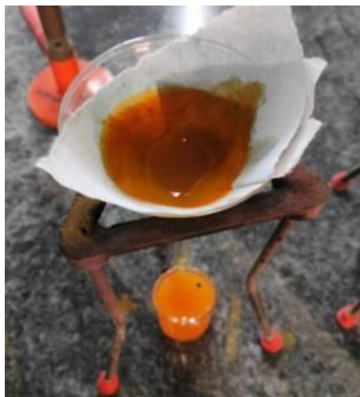
Fig. 7: Filtration of Turmeric Extract.
