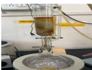
Extract by Soxhlet method
