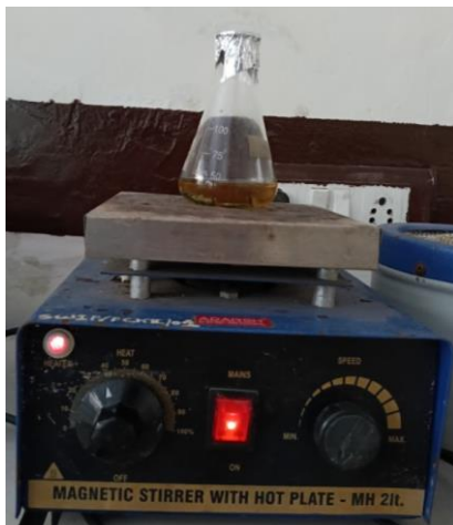
Fig. 5: Emulsification process during preparation of the polyherbal face serum using a magnetic stirrer with hot plate.
