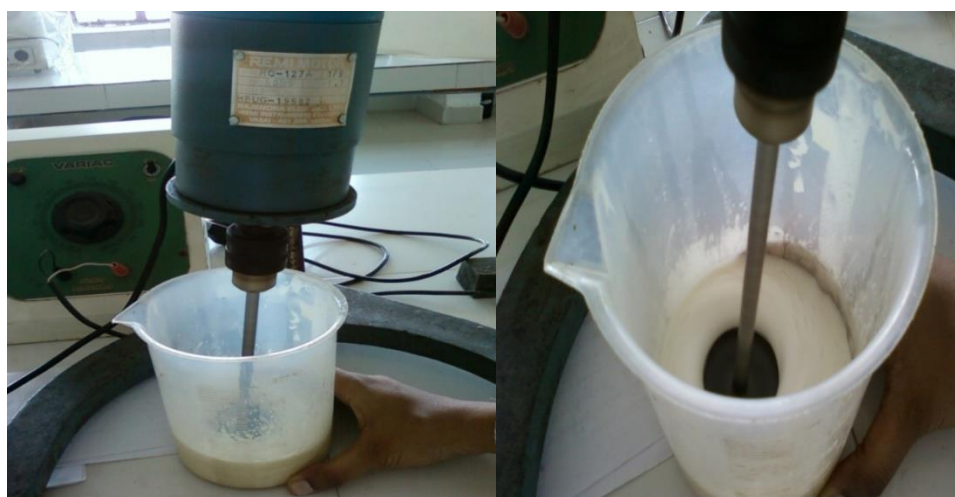
Figure 6.2: Preparation of Floating Microspheres.
