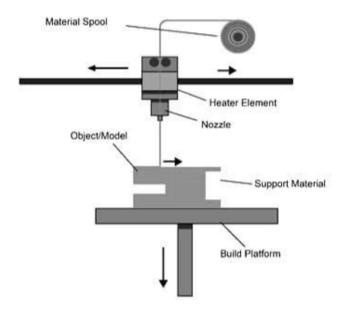
Similar to 3DP, the layout for FDM consists of print head able to move along x and y directions above a build platform. The polymer is extruded through the heated nozzle and laid down as filaments according to CAD design. The build platform is then lowered and another layer can be built, until the scaffold is completed. [23]
