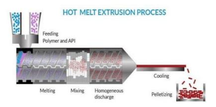
It is a continuous manufacturing technique that involve feeding, heating, mixing and shaping.<sup>[30]</sup> In recent years, it has proved that hot melt extrusion capable to optimise the solubility and bioavailability of moderately soluble drugs.<sup>[31]</sup>
