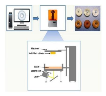
Stereo-lithography requires the use of supporting structures which serve to attach the part to the elevator platform, supports are generated automatically during the preparation of 3D computer aided design model for use on stereo-lithography machine, supports must be removed from the finished product manually, unlike in other, less costly, rapid prototyping technologies.
