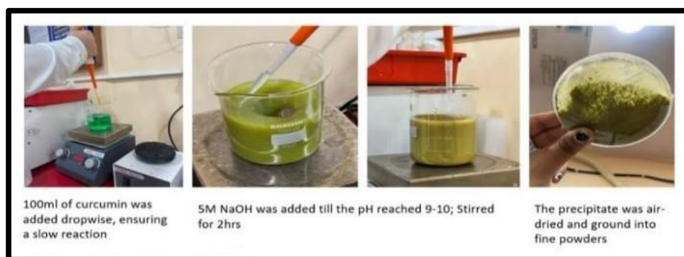
Fig. 1: Curcumin based green synthesis of Nickel nanoparticle.
