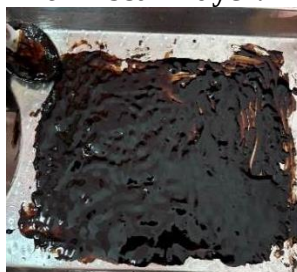
Fig. 5: Scum spread in tray for drying.
