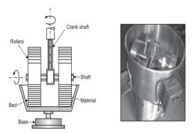
Ball mill<sup>[10]</sup> – Is used to grind the materials to get a course or fine powder. Ball mill principle work on impact and attrition, impact means pressure exerted by two heavy objects, attrition means reduce the size of material when they colloid by heavy weight (ball).
