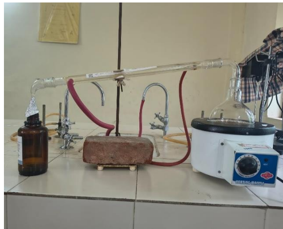
Fig. no. 5: Distillation process.
