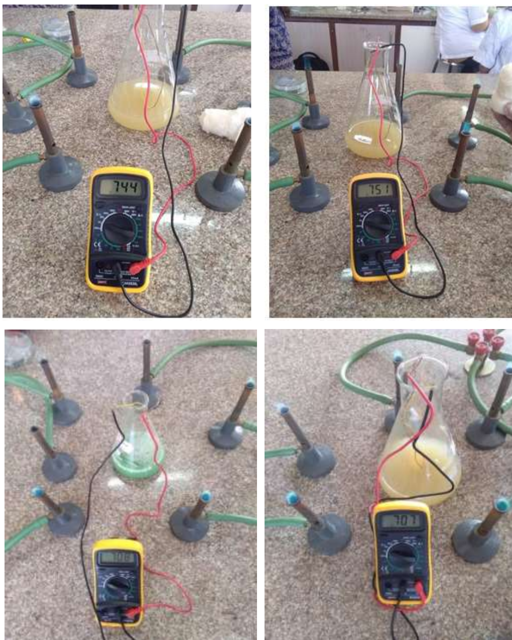
Plate 3.1: Electricity Production by Bacteria in nutrient broth.
