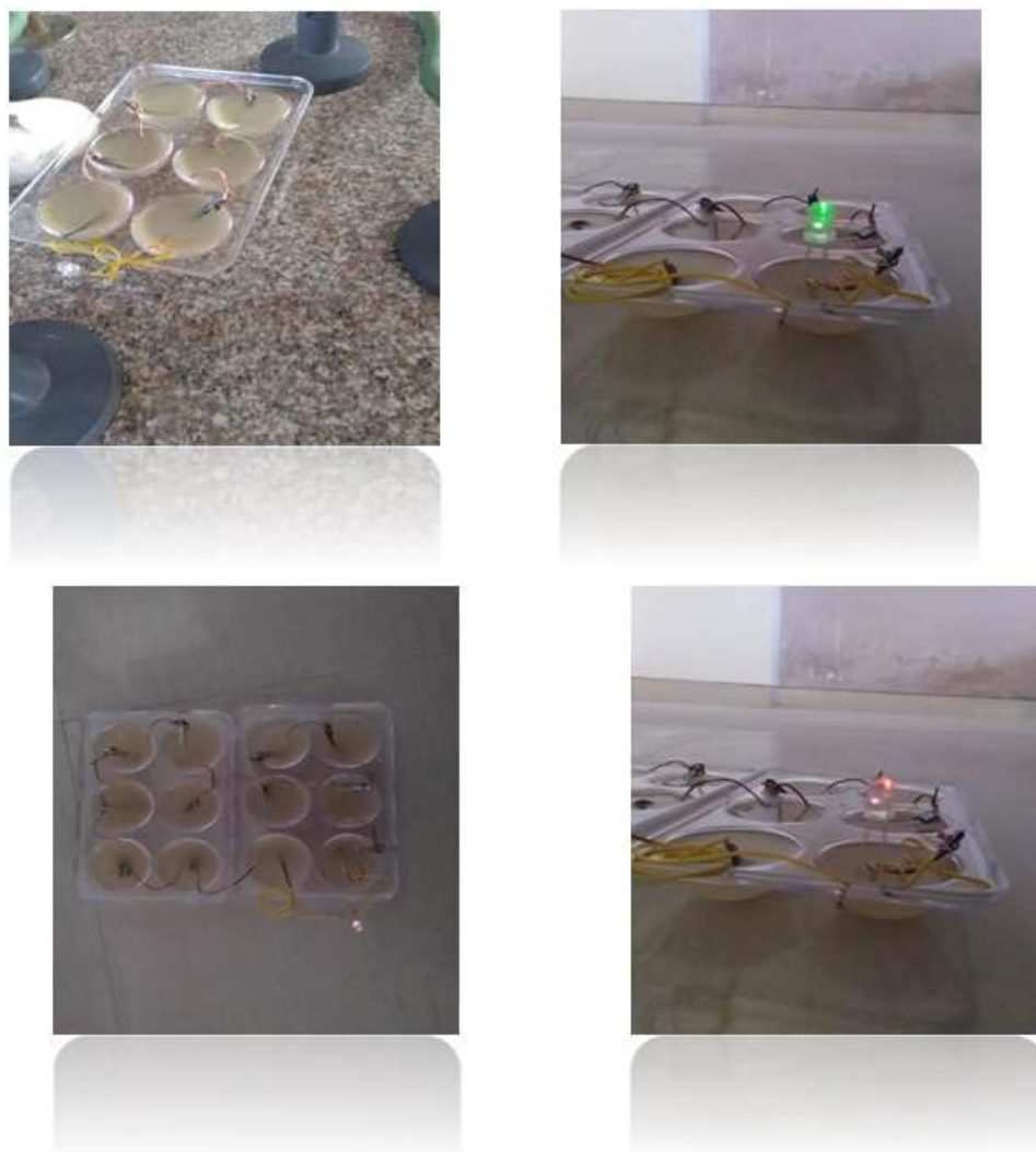
Plate 3.3 Electricity Production by Bacteria
