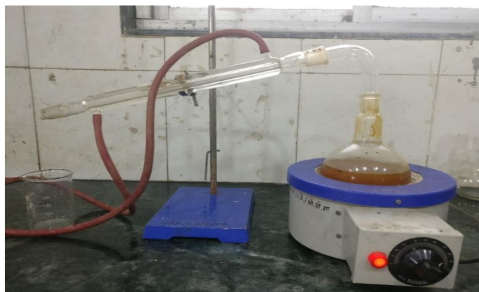
Preparation of dadrunashak arka using distillation apparatus
