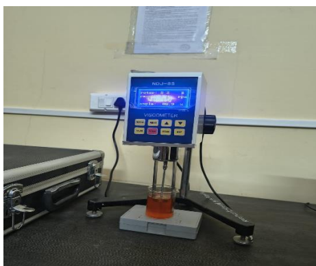
Figure 4: Brookfield viscometer test.
